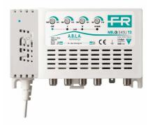
4-input (III+DAB, IV, V, UHF) multiband TV indoor amplifier with 35dB gain and up to 120dBµV output level on UHF band, separate amplification with independent level adjustment (20dB) for each input and low noise figure. T2 technology with UHF cut band for LTE 4G @790MHz and 5G @694MHz.
